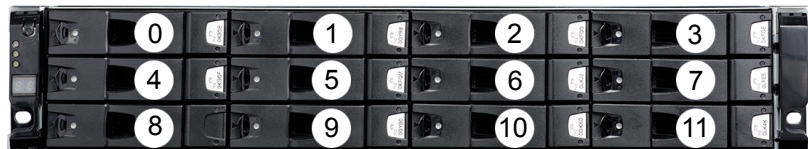
Figure 2-1 2U12 Storage Shelf disk drive slot layout
