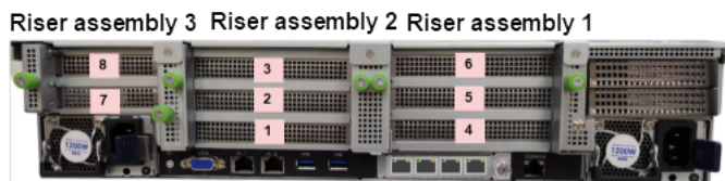
Figure 1-7 Rear panel riser assembly locations and PCIe slot number assignments
