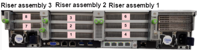
Figure 1-7 Rear panel riser assembly locations and PCIe slot number assignments
