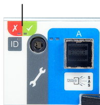
Figure 2-22 Expansion I/O module Status indicator LED location
